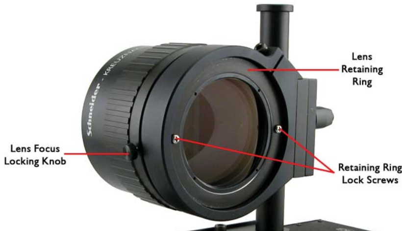
Illustration #2 - Detail of Lens Retaining Ring
